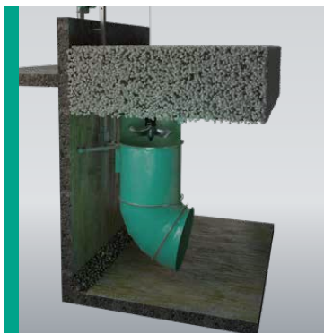
Floating top layer of biomass substrate particles.
