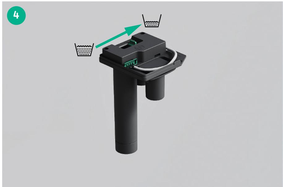
Insert the maintenance unit and fix it with the four screws.
