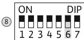
Fig. 14: DIP switch 1: Pump kick
