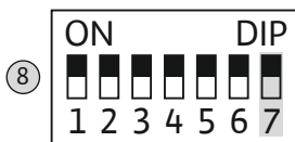
Fig. 13: DIP switch 1: internal buzzer
