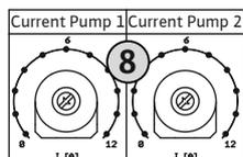
Fig. 5: Set the rated motor current at the potentiometer
