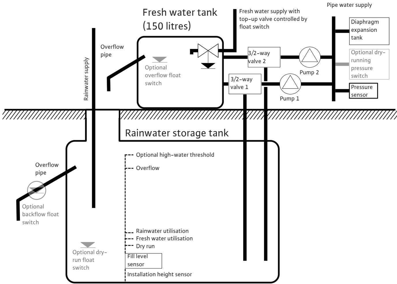
Fig. 20: Functional principle of the AF15 shown schematically
