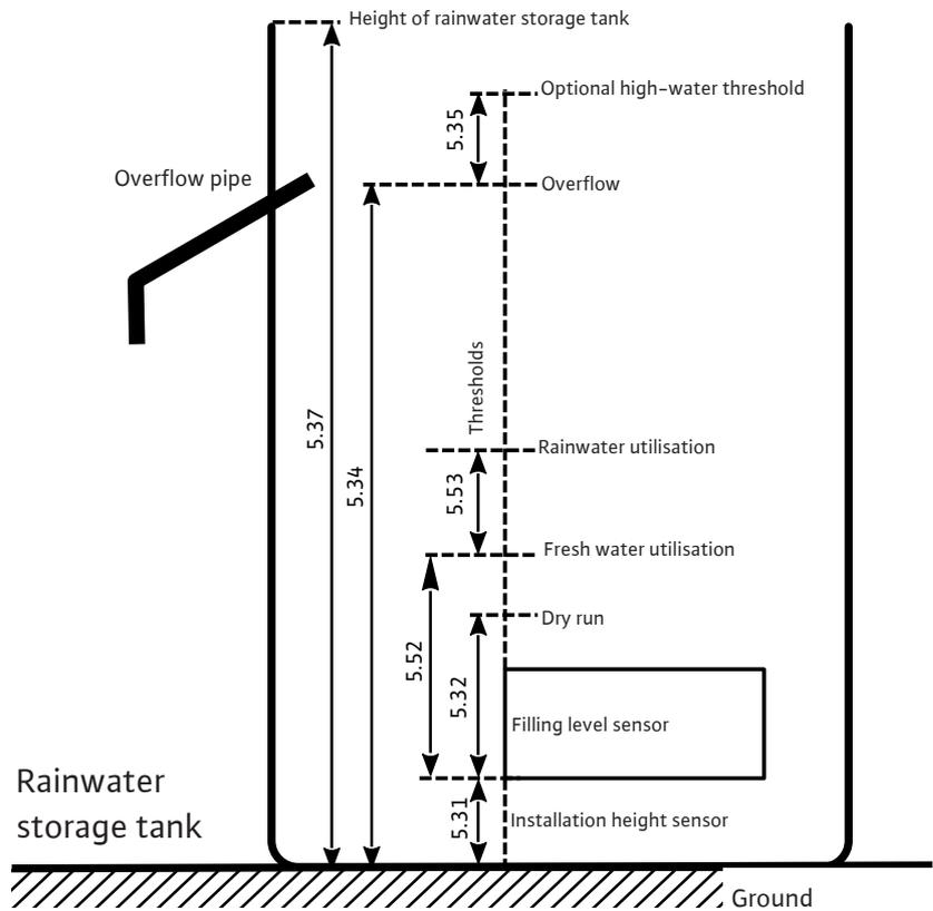
Fig. 21: Setting parameters and menus for the settings
