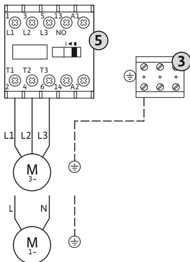
Fig. 4: Pump connection
