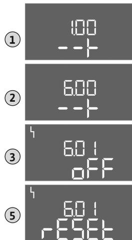
Fig. 115: Acknowledge fault
