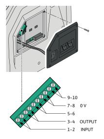
Fig. 6: Extension card connections
