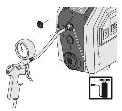
Fig. 14: Filling the diaphragm expansion tank
