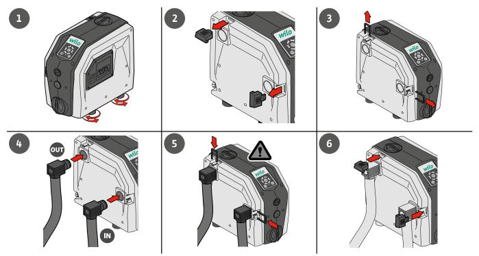
Fig. 5: Hydraulic connection
