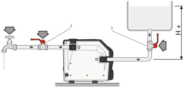
Fig. 12: Load operation
