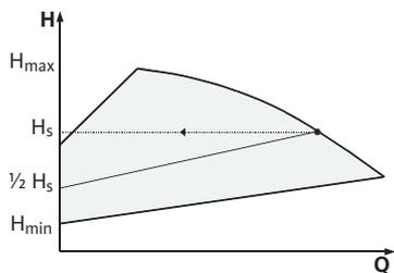
Fig. 7: Modo de regulación  $\Delta p-v$
