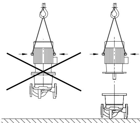
Fig. 2: Transport motora
