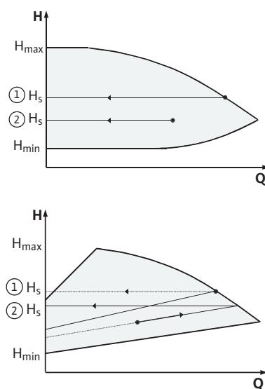
Fig. 32: Regulacija  $\Delta p\text{-}c/\Delta p\text{-}v$
