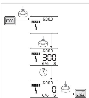
Fig. 54: 确认B型故障 ( $X = Y$ )
