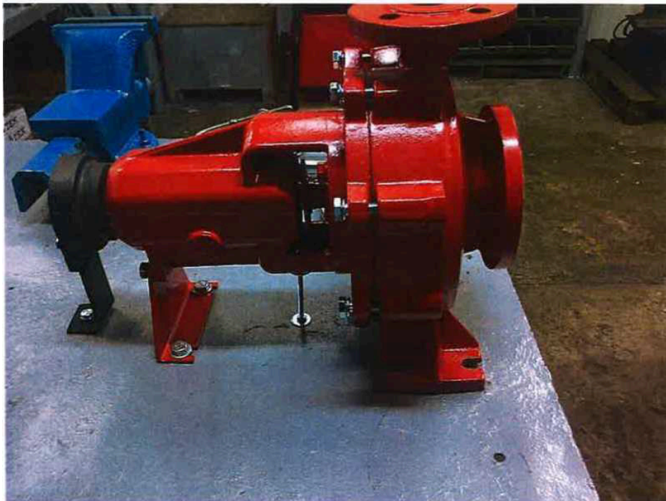
Photograph 3. The firefighting pump type WNF-S 32-250/210-15/2-L1. Source: CNBOP-BIP
