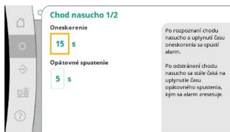
Fig. 36: Bod menu Nastavenia → Nastavenia monitorovania → Chod nasucho 1/2
