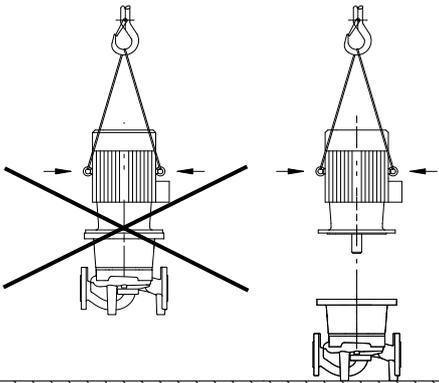
Fig. 2: Transport motora
