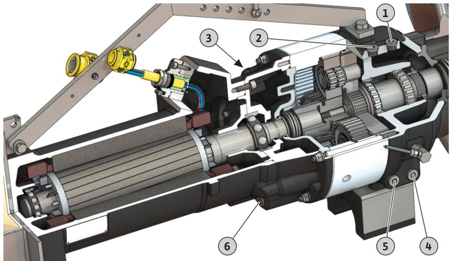
*Fig. 14: Position of the screw plugs*
