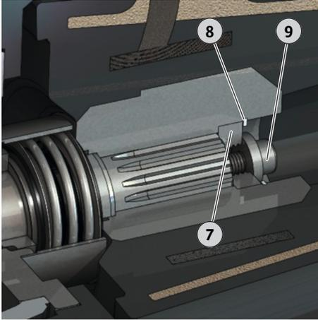
Fig. 17: Propeller attachment
