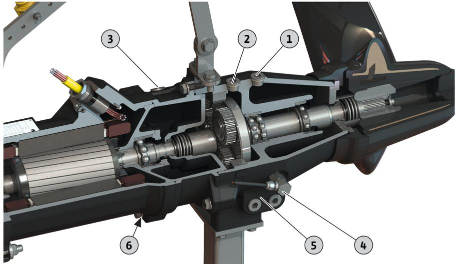
*Fig. 13: Position of the screw plugs*
