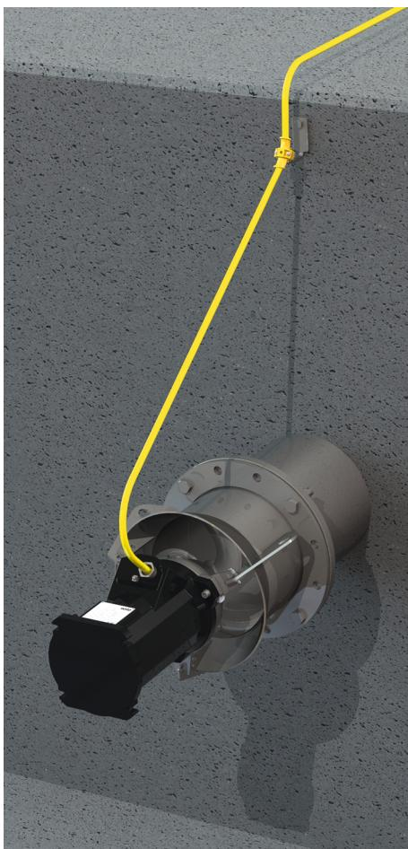
The flow ring is fitted with a flange to screw the recirculation pump to the discharge pipe. Screw the recirculation pump to the discharge pipe using technically approved screws. Installation may **only** be performed when the basin is empty.
