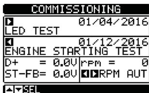
→ From this page, by pressing the key
