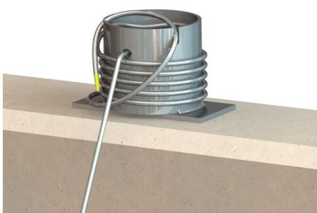
*Fig. 8: Lifting equipment secured with cable bollard*
