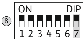
Fig. 16: DIP-bryter 1: intern summer
