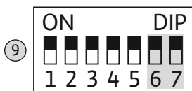
Fig. 10: DIP switch 2: Switch on pumps
