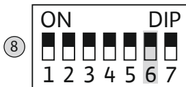
Fig. 17: DIP switch 1: Pump kick
