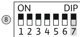
Fig. 16: DIP switch 1: internal buzzer
