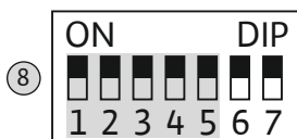
Fig. 9: DIP switch 1: Adjust motor current monitoring
