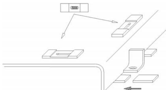
If anchor bolts have been pre-cast in the foundation slightly tighten the anchor bolts. Otherwise let them hang in the foundation holes.
