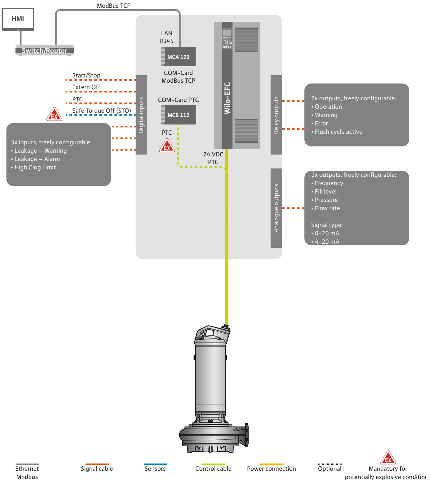
Fig. 14: Connection of LSI system mode: Frequency converter
