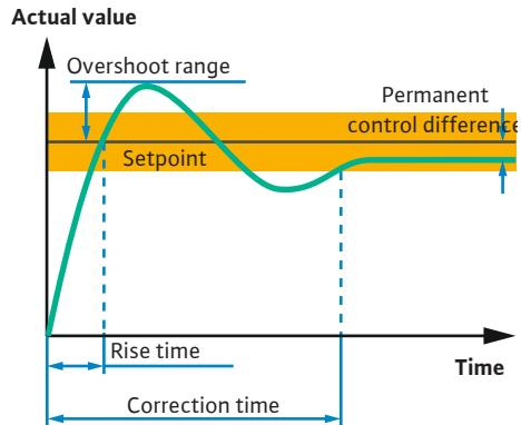
Fig. 17: Step response of a control loop
