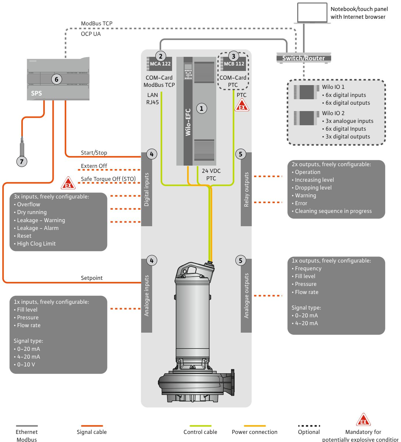
Fig. 4: Installation suggestion with analogue setpoint specifications
