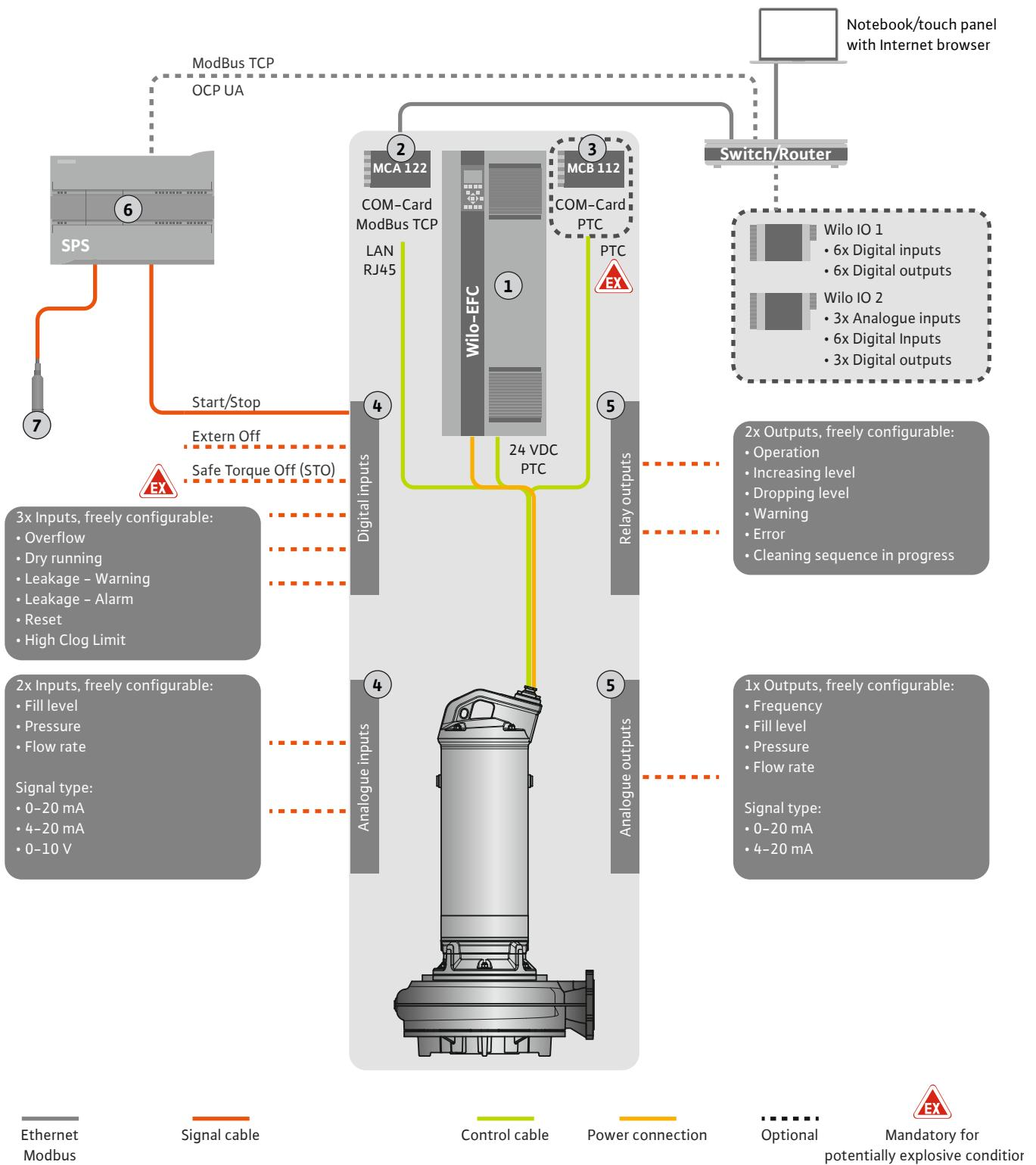
Fig. 3: Installation suggestion with start/stop
