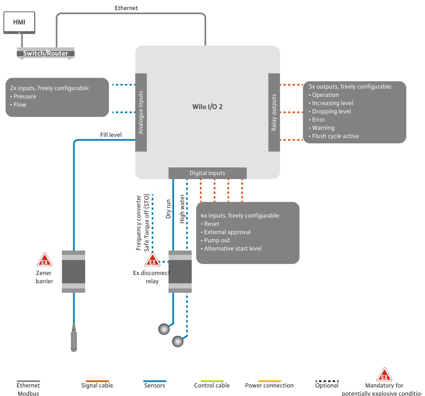
Fig. 13: Connection of LSI system mode: I/O2 module
