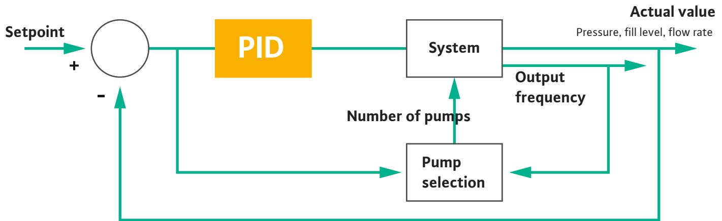
Fig. 15: Control loop with PID controller
