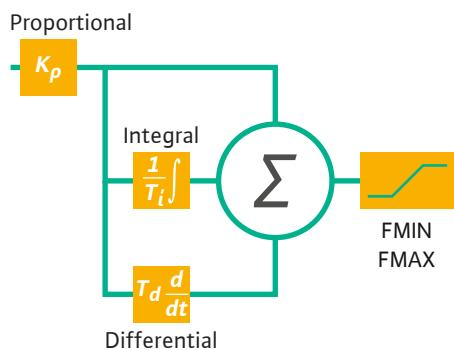
Fig. 16: PID controller
