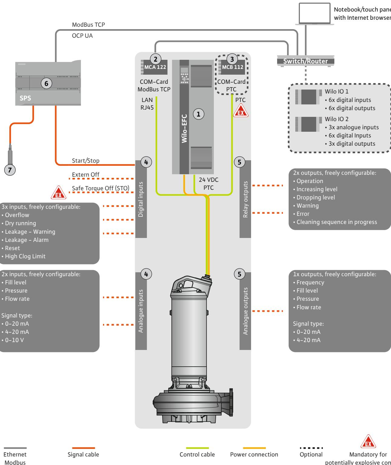
Fig. 5: Installation suggestion with ModBus
