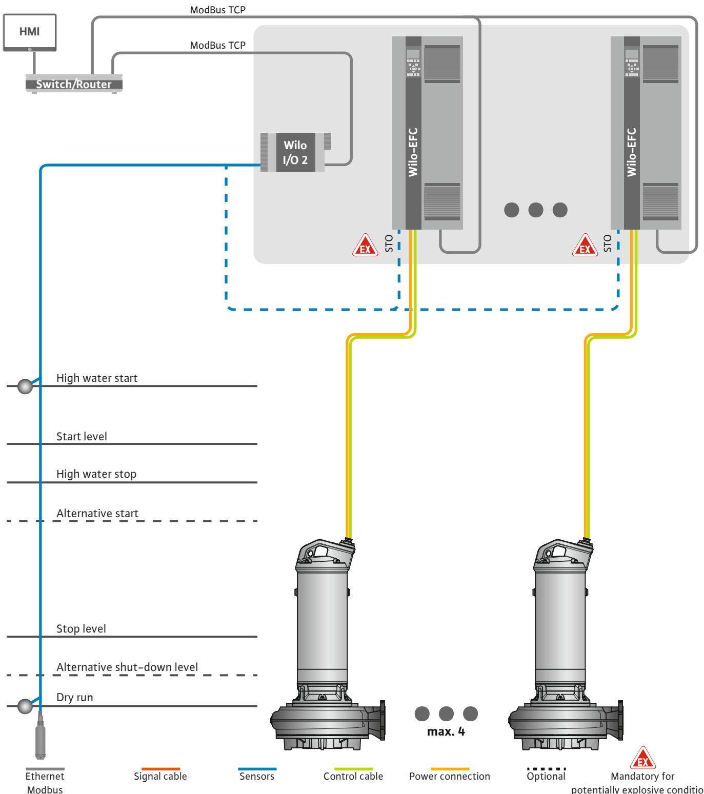
*Fig. 12: Connection of LSI system mode: System overview*
