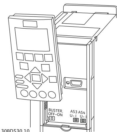
Fig. 9: Position for switches A53 and A54
