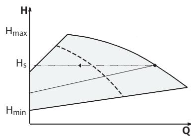
Fig. 15: Regulering  $\Delta p$ -v (paralleldrift)
