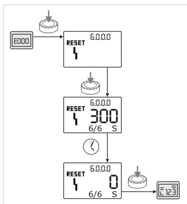
Fig. 48: Conferma del tipo di errore B ( $X=Y$ )**11.3.3 Tipo di errore C**
