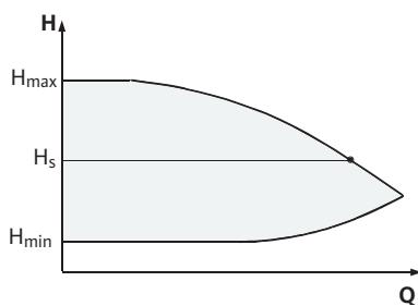
Fig. 10: regulación  $\Delta p$ -c
