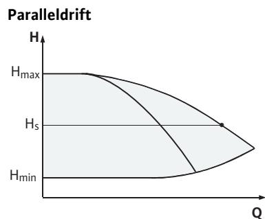
Fig. 14: Regulering  $\Delta p$ -c (paralleldrift)
