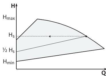
Fig. 11: Regulación  $\Delta p$ -v
