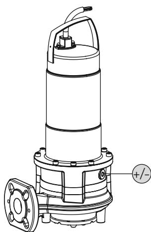
Fig. 4: checking the oil
