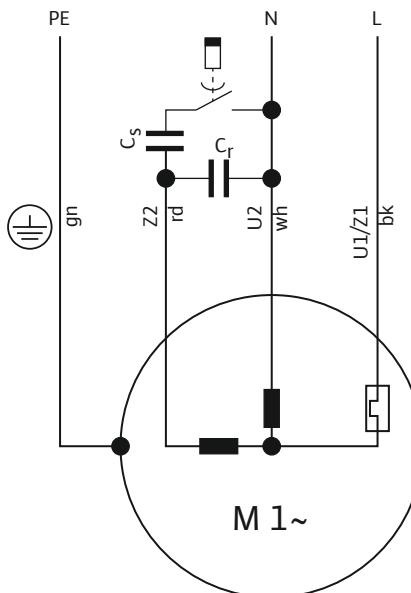
Fig. 7: Connection diagram of the single-phase AC motor
