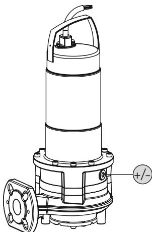
Fig. 9: Sealing chamber: Oil change
