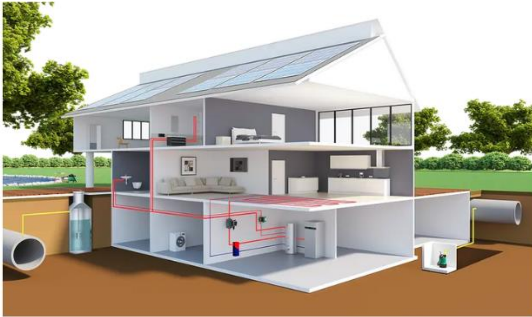
Example of Hydronic Heating and Domestic Hot Water Recirculation in a Closed-Loop System
