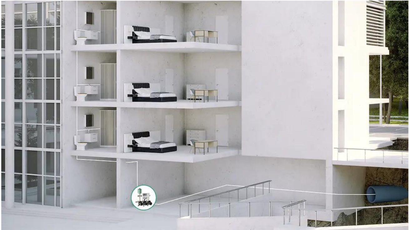
Image 3: An “open system” in a residential building where the water’s final discharge (faucet, toilet, shower, etc.) is “exposed to atmosphere”.
