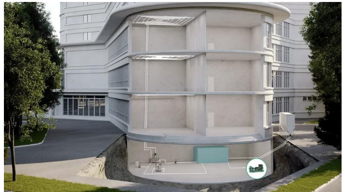
Image 5: A “closed system” to transport thermal energy for heating in a residential or commercial building
