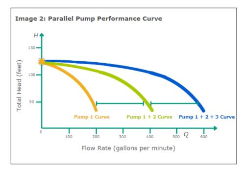
But how does the pump system operate? Pumps operate along the system curve. Even though we have an additive flow with multiple pumps, we will see an increase in flow, but never the total maximum flow due to the system curve.
