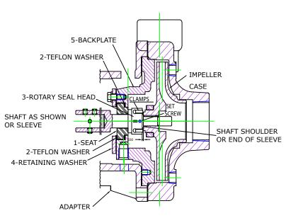
5/8" Seal with stub shaft (shown).
