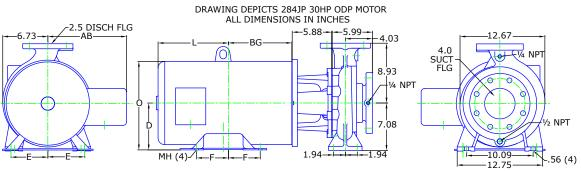
Dimensions are the next larger 60Hz motor derated for 50HZ operation.
