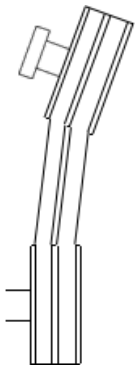
MISALIGNED: SHAFTS NOT PARALLEL
