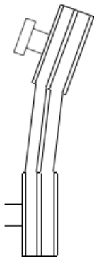
MISALIGNED: SHAFTS NOT PARALLEL
