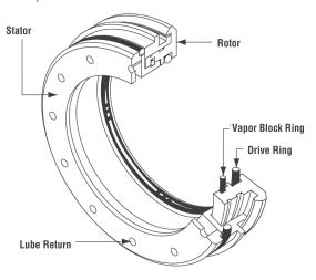
FIGURE 46 - Bearing Isolator
