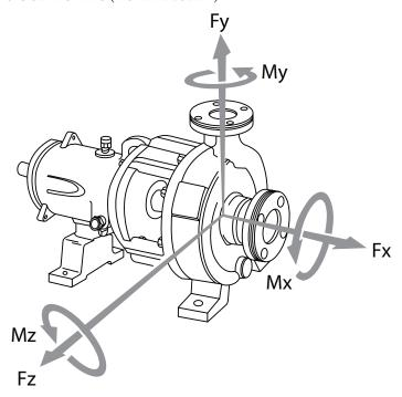
The allowable nozzle loads listed in Figure 52 may be applied to any OSD Standard Horizontal and Lo-Flo pumps in Ductile cast iron, Carbon Steel, 316 Stainless Steel, Cd4MCu, Monel, and Inconel. The allowable loads must be multipled by 0.70 for pumps made of nickel, titanium, zirconium and high chrome iron.
