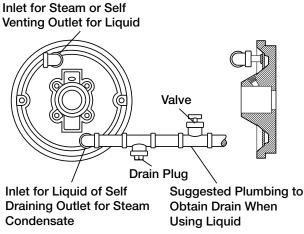
FIGURE 11 - Seal Chamber Cooling
