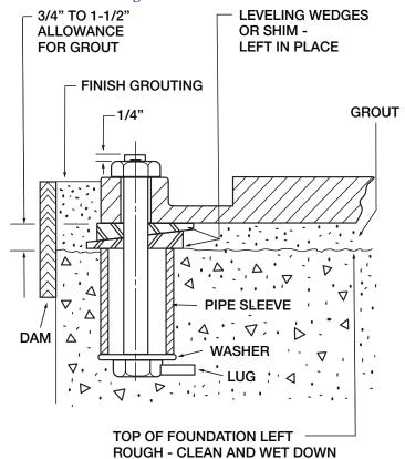
FIGURE 5 – Base Plate Foundation
