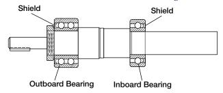
FIGURE 17 - Shielded Bearing Arrangement
