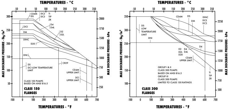
FIGURE 2 – Pressure-Temperature Limits By Alloy
