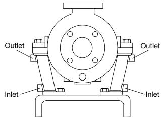
FIGURE 10 - Support Leg Cooling
