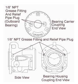
FIGURE 30 - Re-greaseable Configuration
