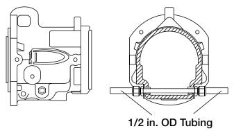
FIGURE 9 – Bearing Housing Cooling
