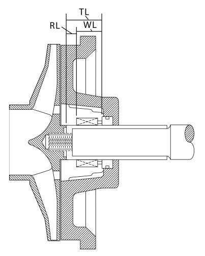
FIGURE 45 - FMI Seal Chamber
