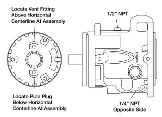
FIGURE 12 - Oil Mist Lubrication - Wet Sump
