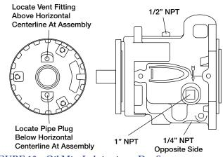
FIGURE 13 - Oil Mist Lubrication - Dry Sump
