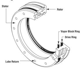
FIGURE 13 - Bearing Isolator
