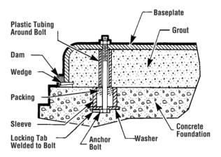
FIGURE 2 - Base Plate Foundation
