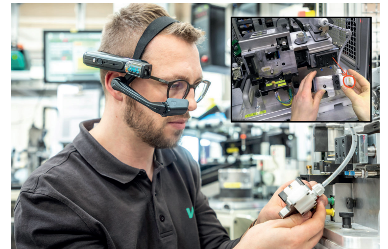
Use of connected glasses for assisting production units
