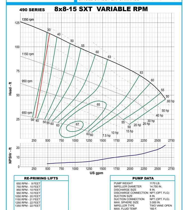
Performance based on pumping clear, fresh water at a temperature not over 85° F., free of gas, air or abrasives and with bowls properly adjusted and submerged. Performance curve reflects Hydraulic Institute tolerances and guidelines.
