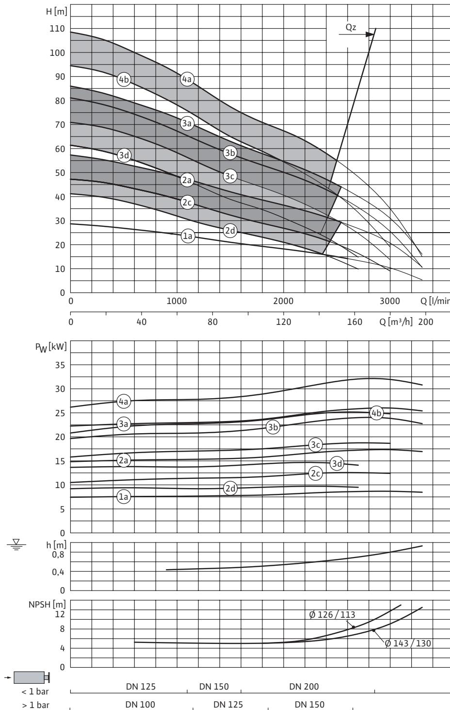
3~400 V, 50 Hz, p = 1 kg/dm<sup>3</sup>, v = 1x10<sup>-6</sup> m<sup>2</sup>/s, ISO 9906 Annex A
