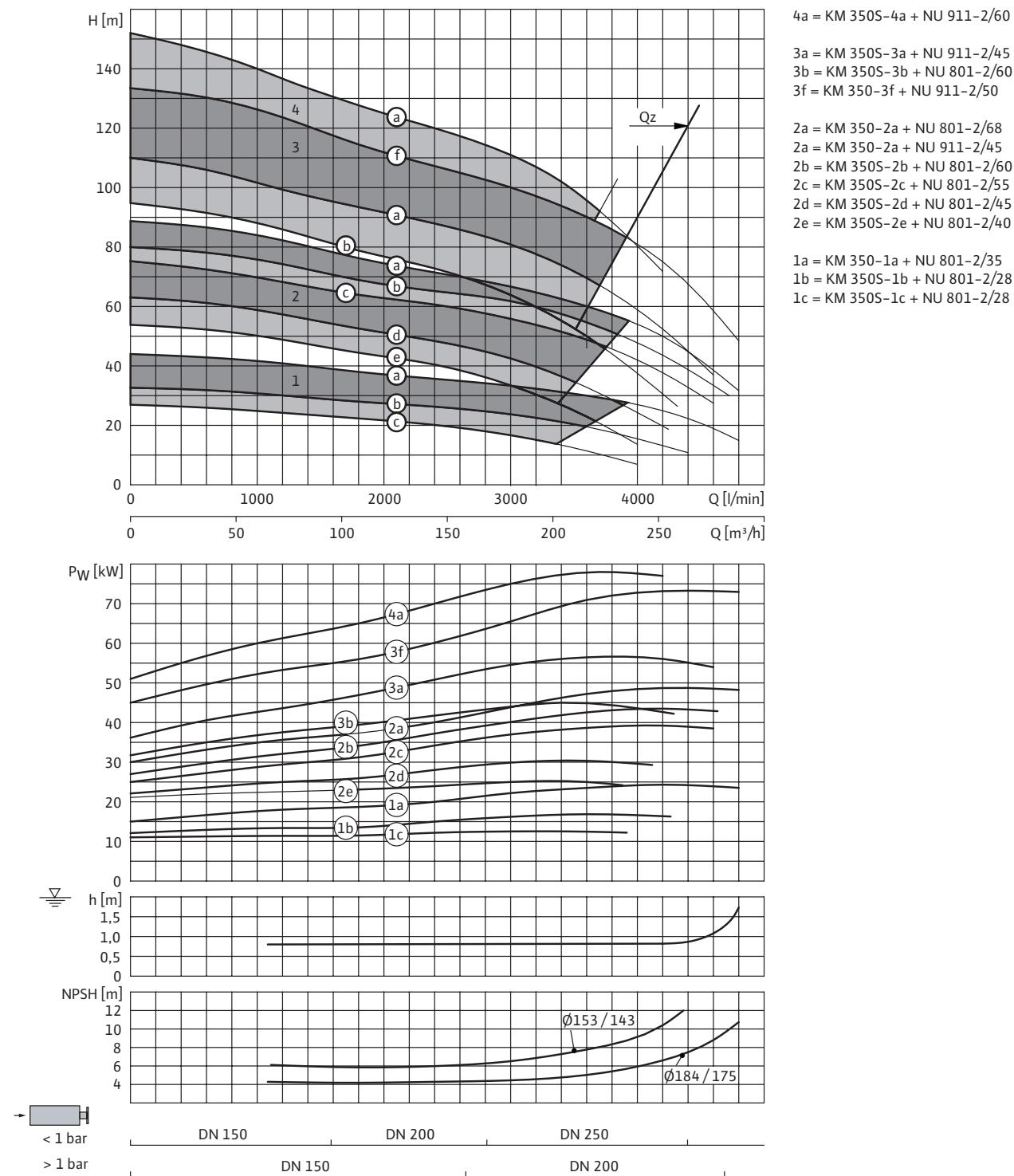
3~400 V, 50 Hz, p = 1 kg/dm<sup>3</sup>, v = 1x10<sup>-6</sup> m<sup>2</sup>/s, ISO 9906 Annex A
