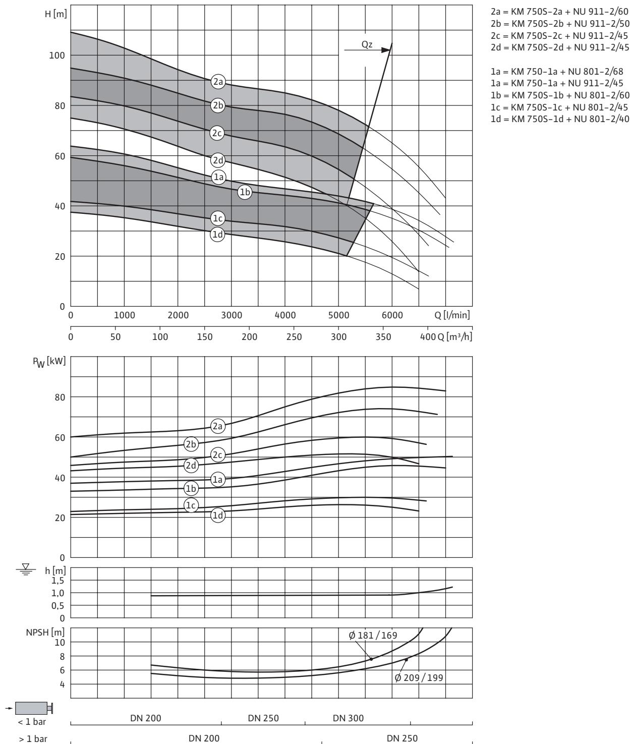
3~400 V, 50 Hz,  $p = 1 \text{ kg/dm}^3$ ,  $v = 1 \times 10^{-6} \text{ m}^2/\text{s}$ , ISO 9906 Annex A
