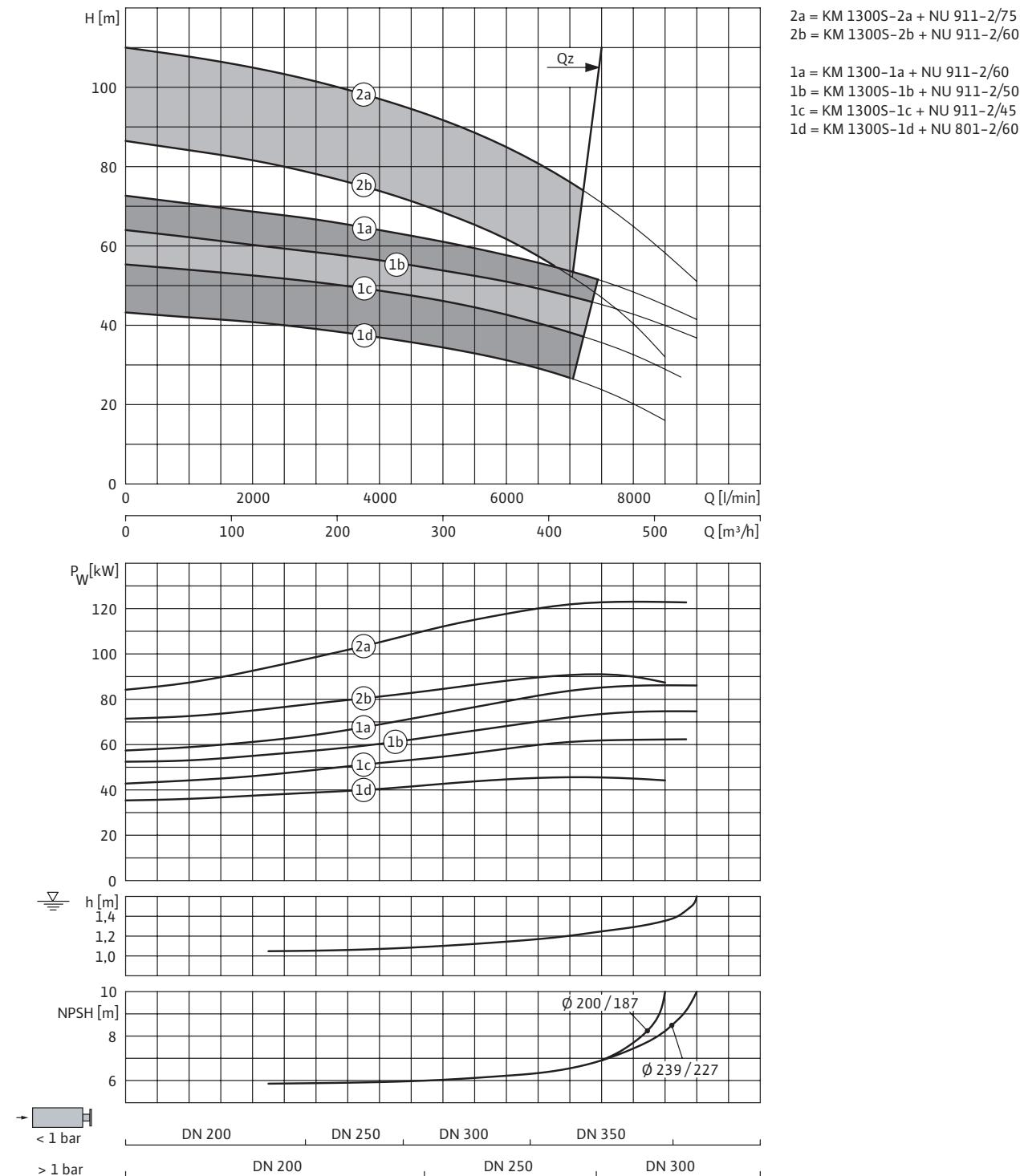
3~400 V, 50 Hz, p = 1 kg/dm<sup>3</sup>, v =  $1 \times 10^{-6}$  m<sup>2</sup>/s, ISO 9906 Annex A
