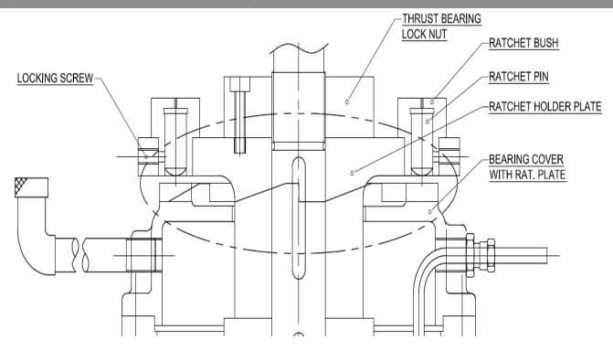
Fig. 15 : Details of Stuffing Box (Page No. 22 & 27, Point No. 5.14 & 8.4)
