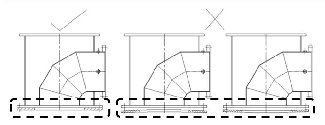
Fig. 8: Support to the discharge piping (Page No. 31, Point No. 8.10)
