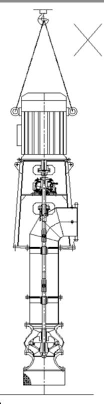
**CAUTION** : Do not lift the Pump with motor Always dismantle the motor before lifting the pump unit.
