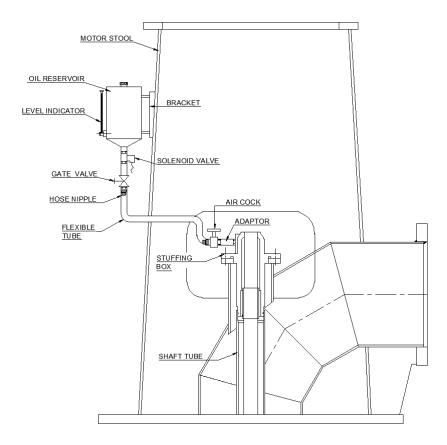
Fig 22: Schematic for forced water lubrication system (Page No. 29, Point No. 8.8)
