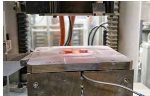
Block magnet production by hot pressing
