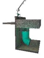
Floating cover of biomass carrier particles
