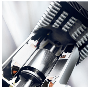
The plastic sealing tube prevents eddy-current losses
