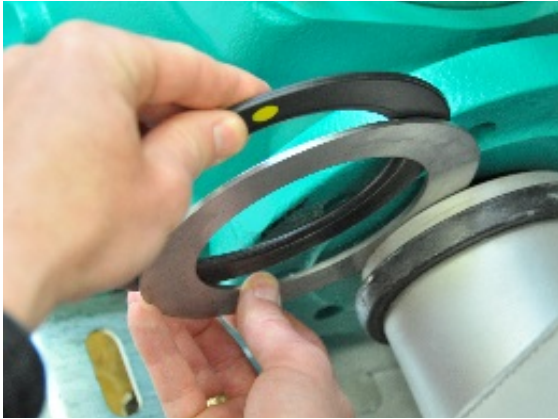
Arrangement of rubber flange gasket and washer.
