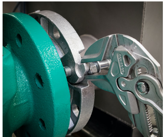
Folding flange rotate opening to secure.
