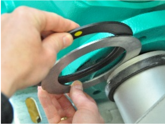
Arrangement of rubber flange gasket and washer.
