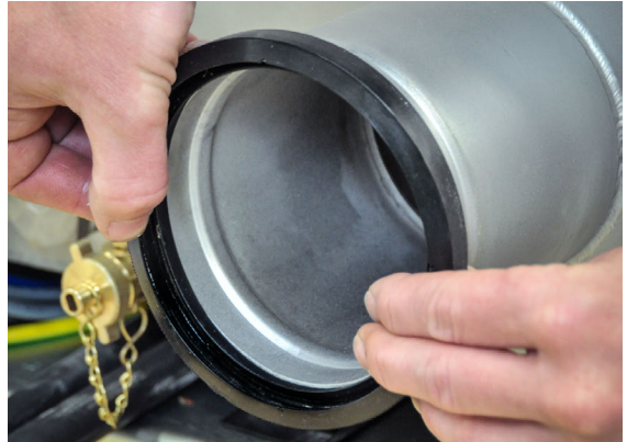
Mount gasket on suction socket.
