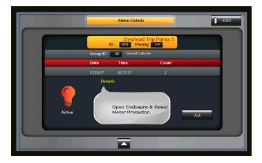
When an alarm is triggered, you will see this screen appear and the alarm horn will sound. You will want to silence the alarm first! To silence the alarm, press the escape key (ESC) which will bring up the alarm log screen.
