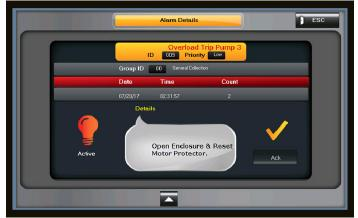
Hit the ESC button three times to return to the main screen.
