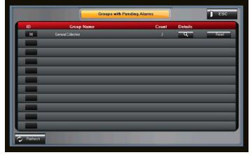
The check mark indicates that the alarm is acknowledged. The red light indicates the alarm is currently active, and the grey light means that the alarm has cleared, but has not yet been acknowledged. Default value is that alarms do not require acknowledgement to reset, except for the pipe burst alarm.
