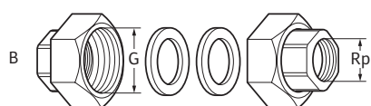
Fig. A: Special union inserts with Whitworth male thread (DIN EN 10226-1) and female thread for choice between threaded connections and solder joints on copper pipe (DIN EN 1057)
