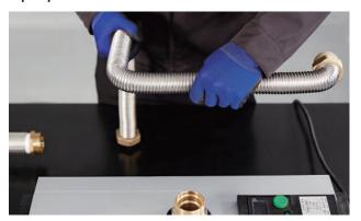
Connecting the wrinkling pipes right after the assembling a valve socket at Suction & Discharge parts
