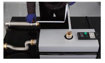
5 Preparing the suitable size of wrinkling pipe to connect the pump.
