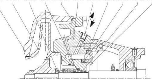
Single mechanical seal + external flushing :
