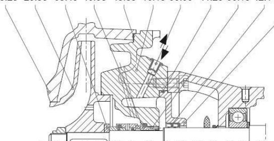
Single mechanical seal + back cover heating :
