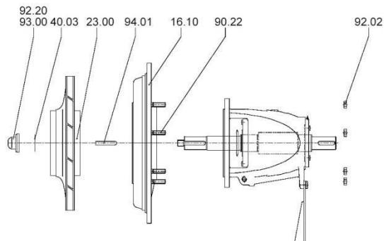
13. Add flat gasket 40.01, key 94.01, impeller 23.00 and flat gasket 40.03.
