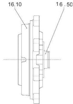
8. Assemble bearing bracket housing 33.00 and casing cover 16.10.
