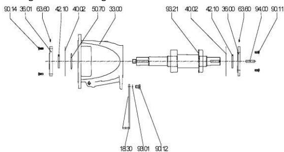
5. Withdraw the shaft with the two ball bearings 32.10 and spacer rings 50.50 and circlip 93.21.
