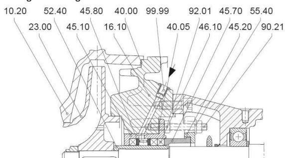
**12.1.1.2 BEARING BRACKETS 55-65 :****Shaft sealing with mechanical seal :**
