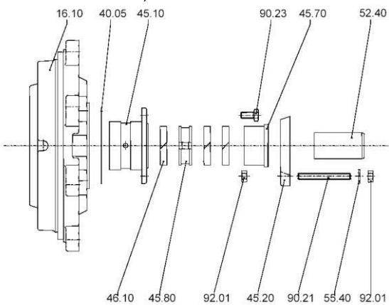
11. Install the pressure ring 45.70 and the gland 45.20. Put the washer 55.40 on the stud bolts and fasten nuts 92.01.
