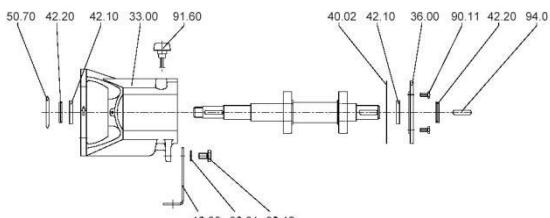
6. Fasten foot 18.30 and slide the thrower 50.70 onto the shaft.
