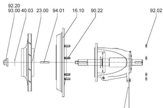
4. Remove impeller nut 92.20 and its helicoid 93.00.
