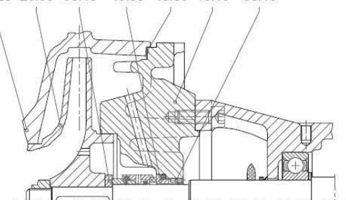
Single mechanical seal + external quench :
