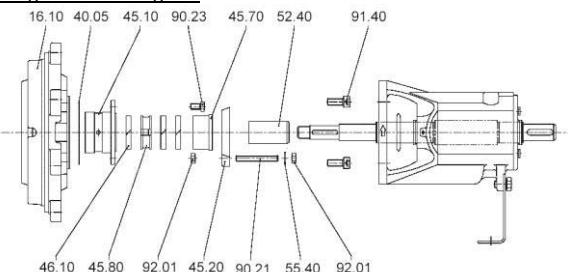
1. Remove the screws 91.40 and remove the casing cover 16.10.
