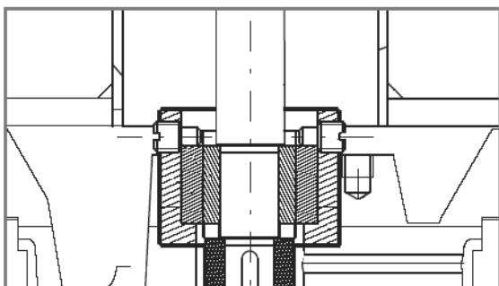
Other bearings are installed in intermediate flanges to guide pump rod correctly.
