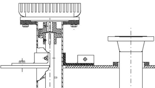
VEM : cast iron pedestal between base plate and motor flange. This assembly allows powers up to 18,5KW. No possible adjustment of pump height. Coupling is direct type between motor shaft and pump rod.
