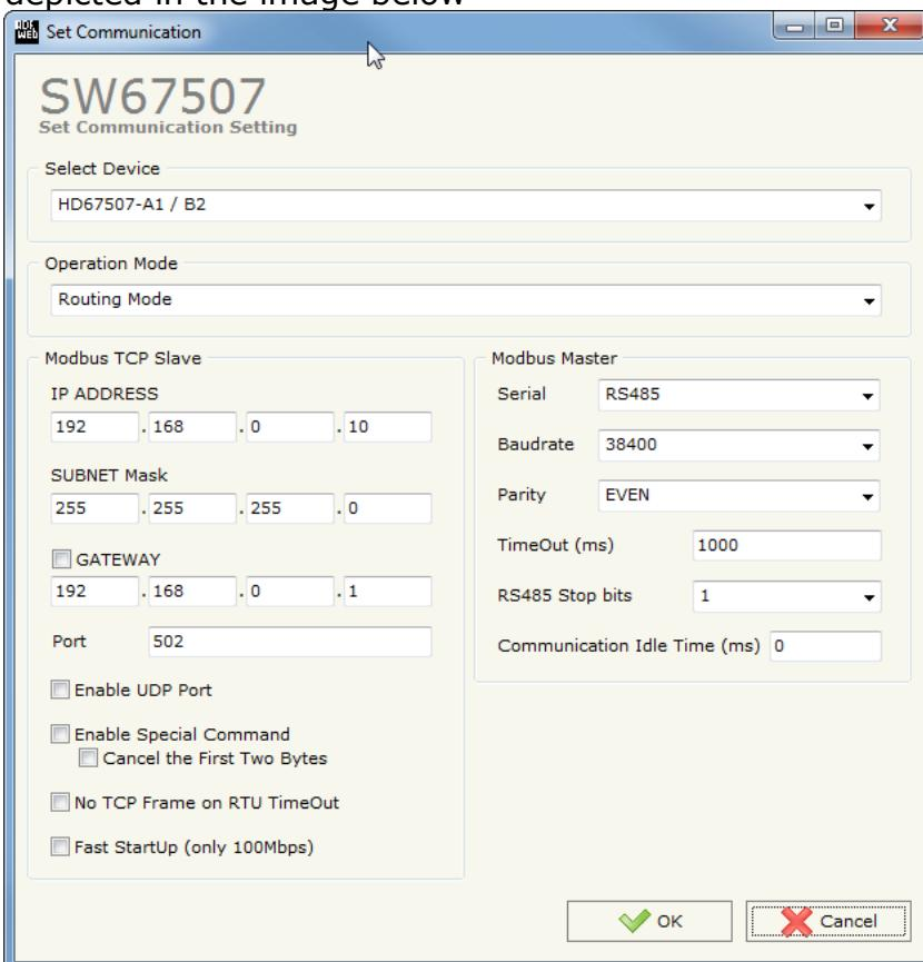
4. The IP address can be change according to the requirements of the network site
