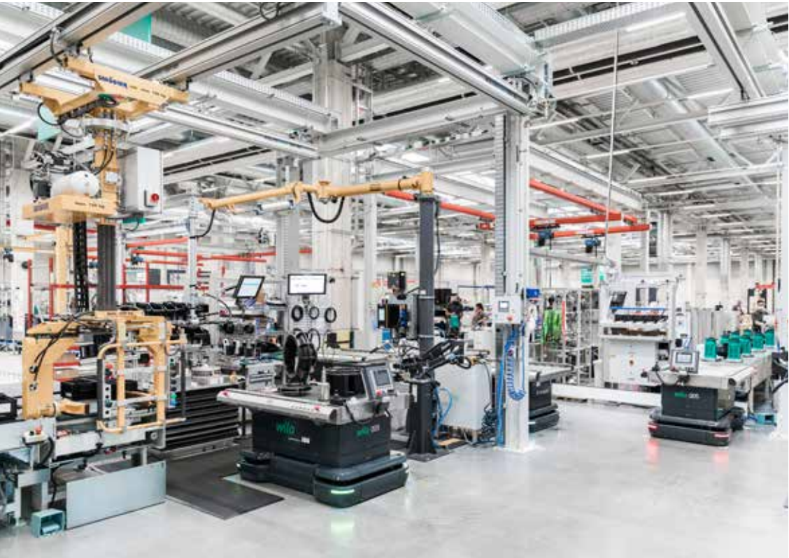
Production at the Wilo smart factory. Automated guided vehicles (AGV) are also incorporated into the intelligent processes. They are used to transport material and support production.
