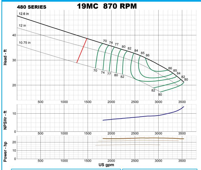
IMPELLER NUMBER0353TYPEENCLOSEDTHRUST FACTORK=32.00EYE AREA74.5 SQ. IN.WEIGHT54.00 LB.
