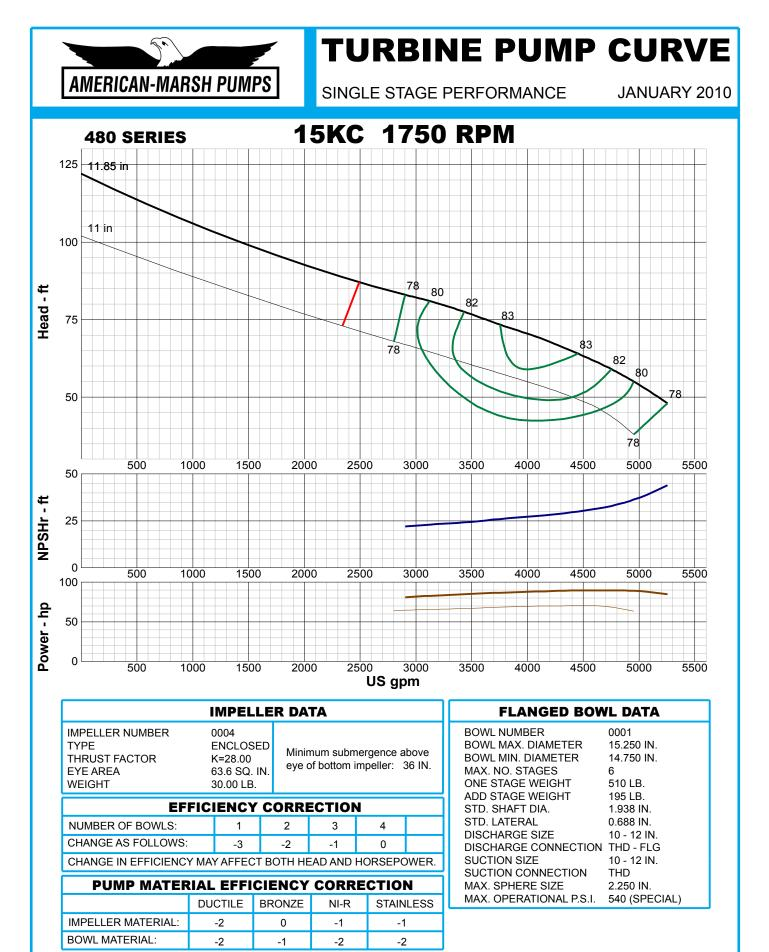
Performance based on pumping clear, fresh water at a temperature not over 85° F., free of gas, air or abrasives and with bowls properly adjusted and submerged. Performance curve reflects Hydraulic Institute tolerances and guidelines.
