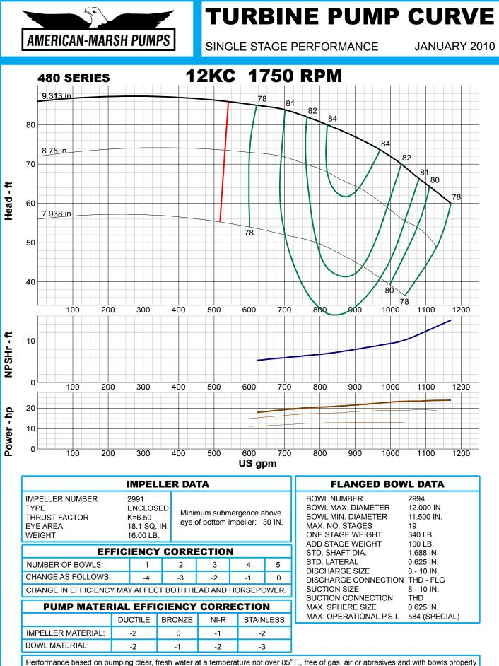
adjusted and submerged. Performance curve reflects Hydraulic Institute tolerances and guidelines.
