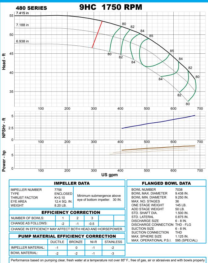
Performance based on pumping clear, fresh water at a temperature not over 85° F., free of gas, air or abrasives and with bowls properli adjusted and submerged. Performance curve reflects Hydraulic Institute tolerances and guidelines.
