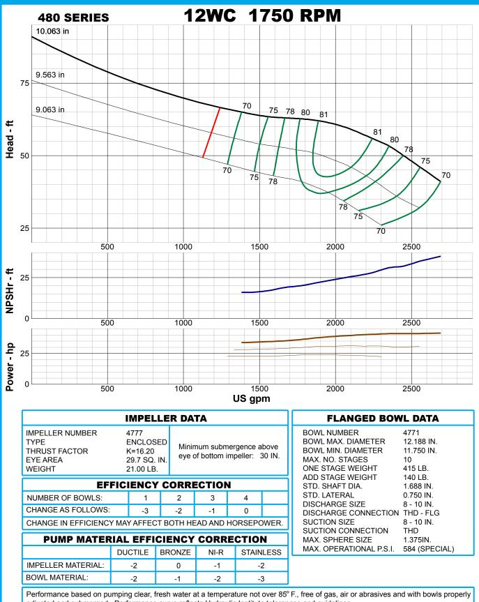
adjusted and submerged. Performance curve reflects Hydraulic Institute tolerances and guidelines.
