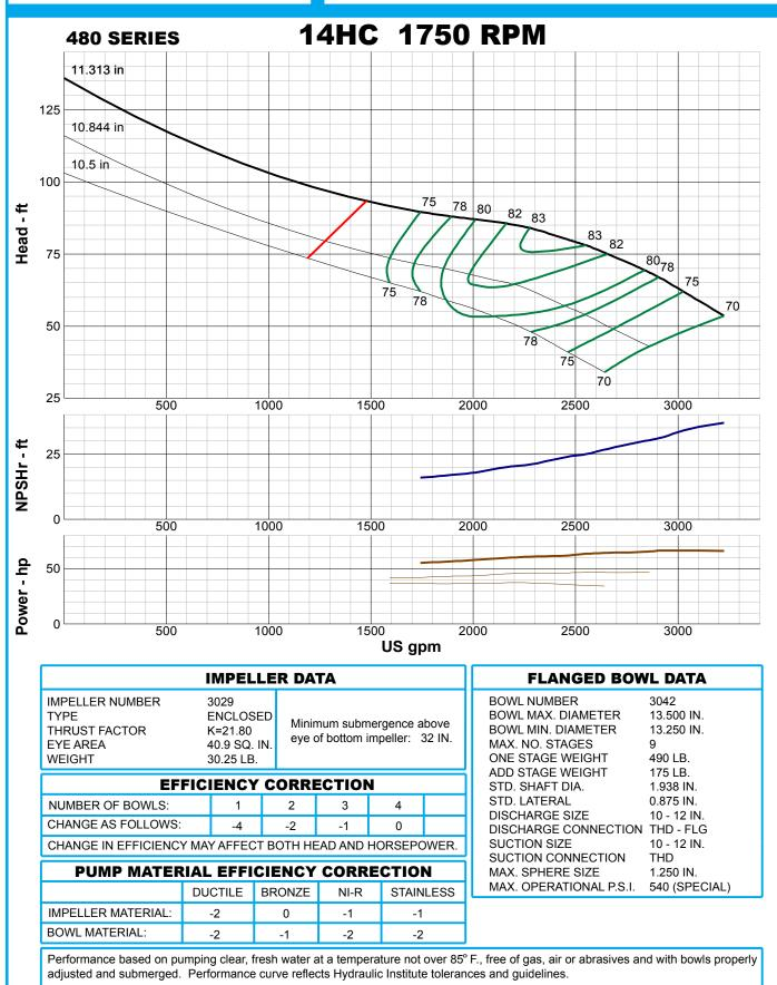
**TURBINE PUMP CURVE** AMERICAN-MARSH PUMPS SINGLE STAGE PERFORMANCE **JANUARY 2010** 14HCR 1750 RPM **480 SERIES** 11.5 in 10.875 in 10.406 in Head - ft NPSHr - ft
